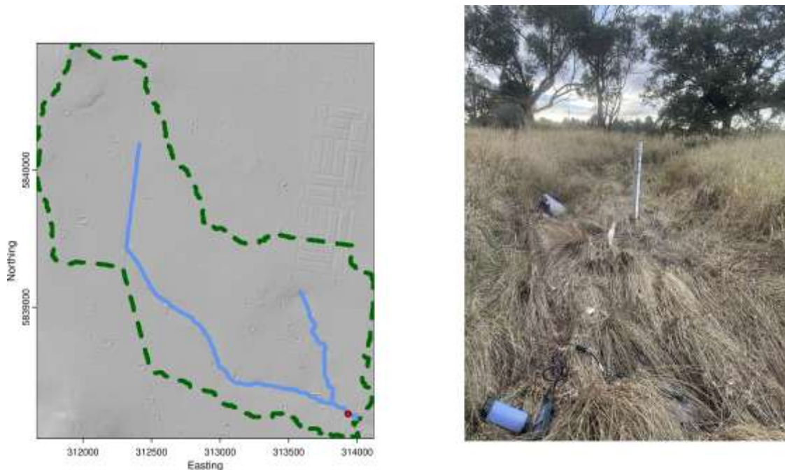
Figure 6: Site map for Aitken Creek (west branch, HTC_340) (left). Dark green dotted lines = catchment boundary. Headwater stream extension lines shown in blue. Monitoring point = red circle. The background is a grayscale representation of the terrain surface (hillshade). Photo of the site shown on the right
